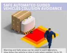
Warning and Safe areas can be used to warn operators, slow down the vehicle or stop it only when needed. Up to 70 different area sets can be configured and activated depending on position, speed and movement of vehicle.
